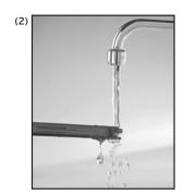
2. Rinse the sensor in clean water and shake off the droplets of water (do not use a cloth).
