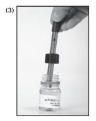
3. Plunge the sensor into the bottle of "mV465" buffer solution.
